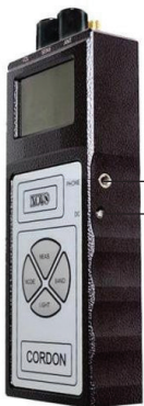
Pic.3. Jacks for headphones and AC/DC adapter.
